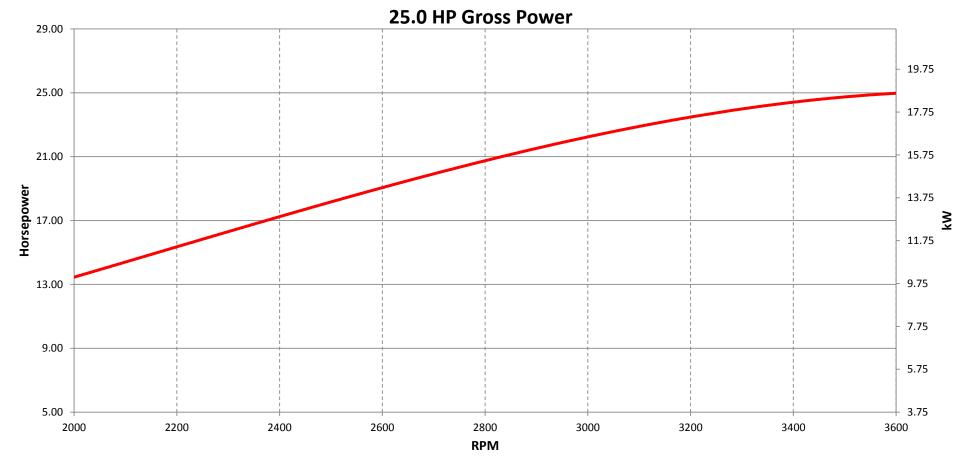
Power Ratings: The gross power rating for individual gasoline engine models is labeled in accordance with SAE (Society of Automotive Engineers) code J1940 Small Engine
